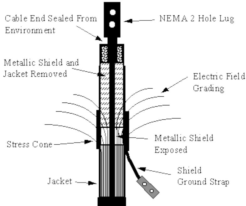
Figure 1 - Typical Stress Relief Cone Shown Electric Field Grading
