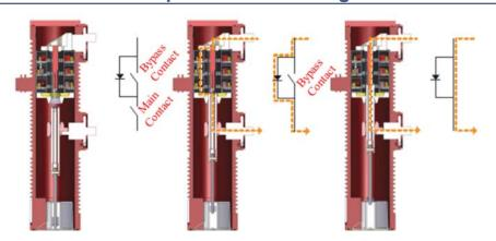
ABB's DS1-M transient free capacitor Switch uses advanced diode switching technology to eliminate problems that once plagued motor start capacitor banks. By exploiting the natural commutation characteristic of a diode, it carries out closing operations without any transient current, voltage, frequency, or possibility of prestrike.
