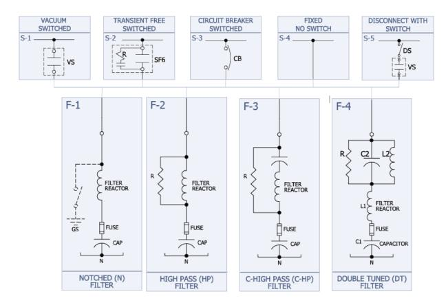
Harmonic filters and capacitors are connected in a number of different ways depending upon bank rating and protection requirements. Typically, harmonic filters are provided with an ungrounded wye or ungrounded split-wye connection, but a grounded wye and Delta connection are also available.
