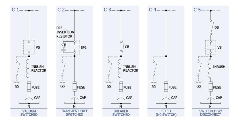
The capacitor bank can be connected in a number of different ways depending upon bank rating and protection requirements. Typically, capacitor banks are provided with an ungrounded wye or ungrounded split-wye connection, but a grounded wye and Delta connection are also available.
