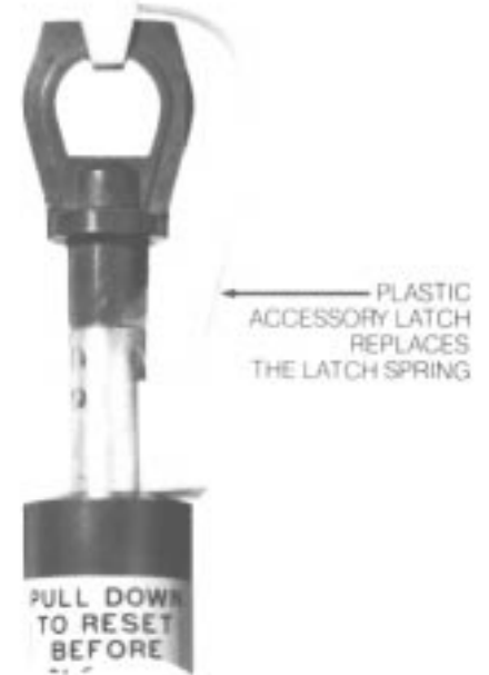
Figure 15. Arc-Strangler loadbreaking device with optional accessory latch.
