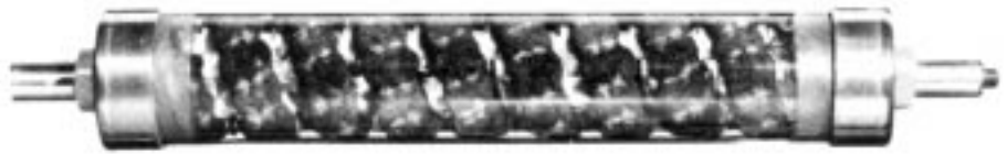
Figure 10. Fulgurite information caused by a high-fault current.
