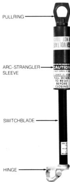
Figure 16. The Cooper Power Systems Arc-Strangler switchblade. (The Arc-Strangler sleeve quickly extinguishes the arc in exactly the same manner as when used on NX fuses.)
