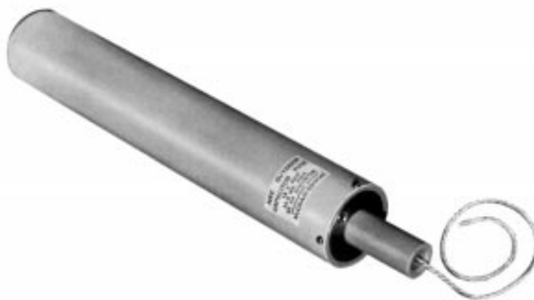
Figure 1. NXC outdoor capacitor fuse, available in voltage ratings of 8.3, 15.5 and 23 kV, offers positive leader wire ejection for reliable interruption and elimination of electrical stress to circuit apparatus. Top end cap has provision for convenient bus bar mounting.
